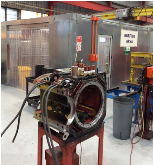
Buffing booth: this isolation area addresses both noise and dust.
