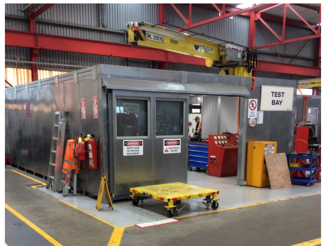
Test Bay: Traction motors are now run in this booth after being overhauled.
